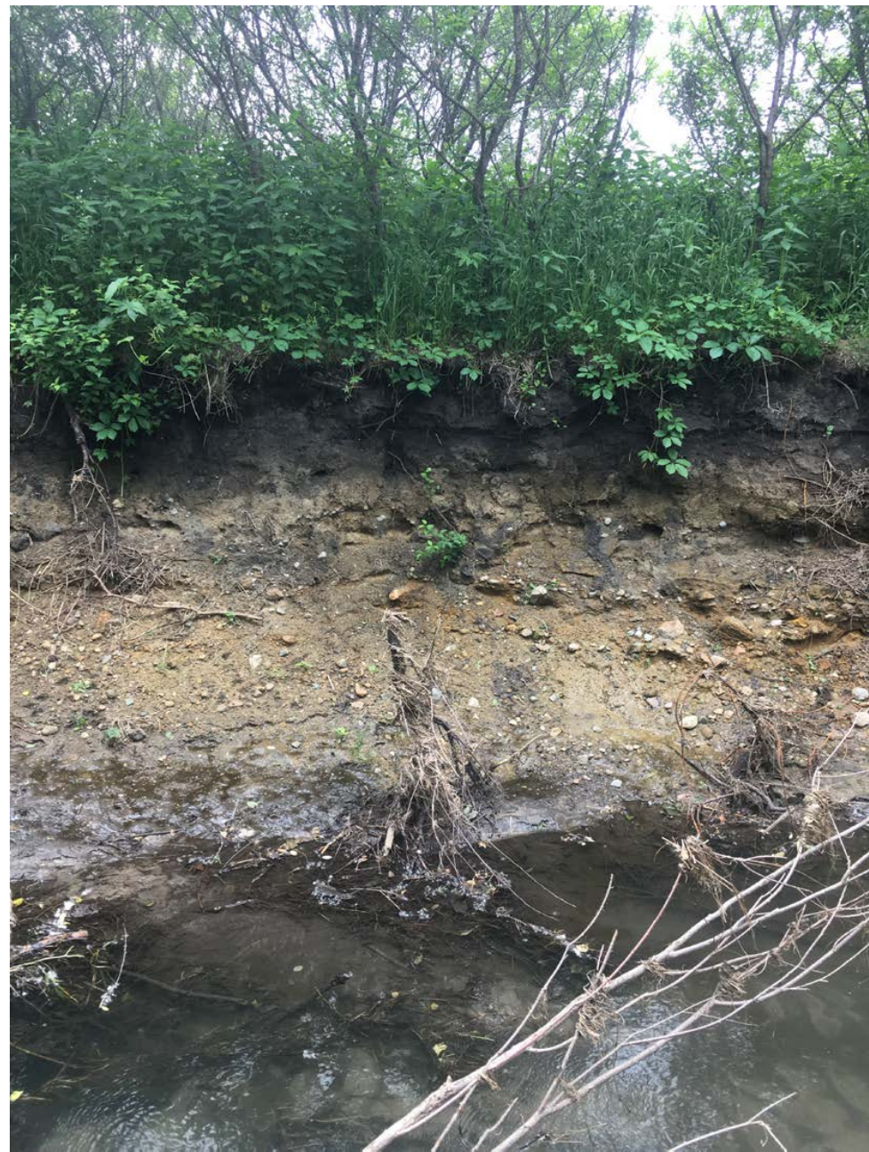
Figure 5. Typical bank soil profile showing top soil, sandy soil, and clay with gravel at the toe in this case.
